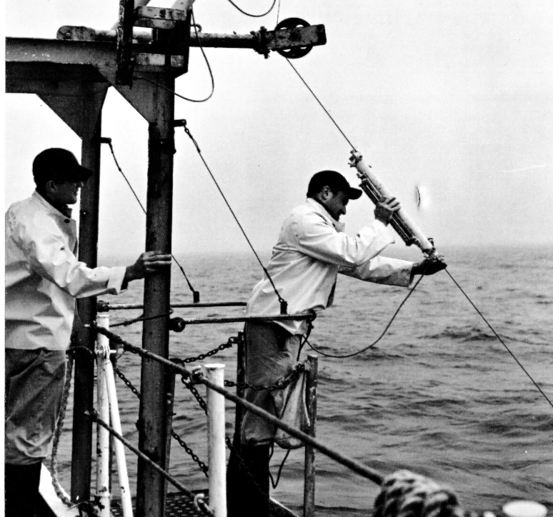
ATTACHING A NANSEN bottle to a cable. Nansen bottles, named for the Norwegian explorer, are used to collect water samples.
