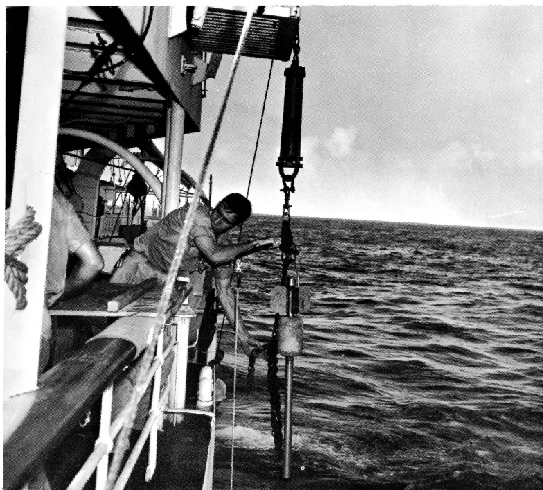
A CORING DEVICE being lowered. This is used to bring up layers of sediment from the ocean floor.
