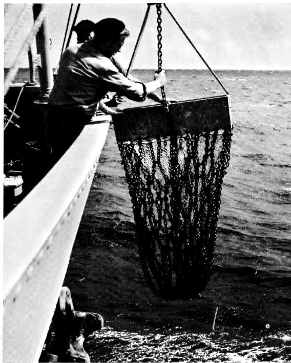
A GEOLOGICAL chain-mesh dredge going over the side. The dredge collects rock samples.
