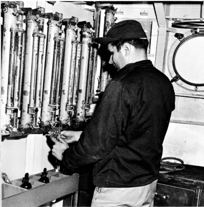
WATER IS DRAWN from a Nansen bottle for analysis.
