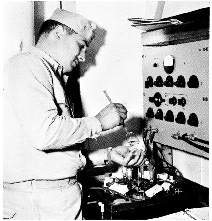
AN OFFICER determines the salt content.
